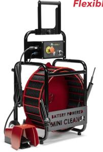
The Picote Mini Cleaner was specially designed for plumbers working in smaller diameter pipes. Thanks to its highly flexible 1/3" shaft, working in  $1\frac{1}{4}$ -3"pipes is extremely easy, even those with multiple  $90^{\circ}$  bends and p-traps as small as 2".
