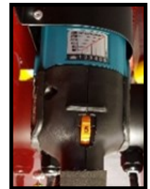
Speed selector located on motor
