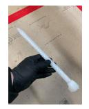
2. Slide retaining nut onto mixing tip.
