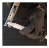
3. Cut off mixing tip at first tier. Use pliers tip to slightly widen the end of the delivery hose. Slide the delivery hose fully over the mixing tip's next tier.
