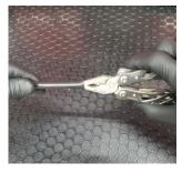
4. Use the tip of needle nosed pliers to slightly widen the end of the delivery hose. Slide the delivery hose fully over the mixing tip tier.
