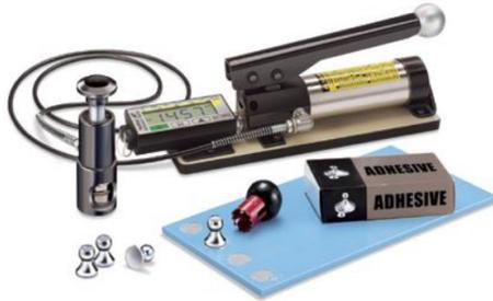
This test can look for two different outcomes depending upon the substrate used. When a brick or concrete substrate is used in a real-world application, it is testing whether or not that substrate breaks before the coating (product) does. If steel were to be used, however, the coating will always break before the substrate, so the PSI is also measured at the time of the break.
