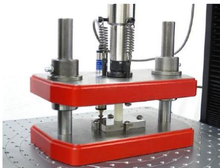
A sample of the product at approximately .25-inches is laid flat and a machine pushes down on the specimen until it begins to compress. The PSI it requires to shear the sample is its “**Compression Strength**”. The amount it swells when the pressure is applied is also measured.
