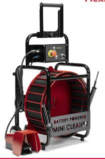
The Picote Mini Cleaner was specially designed for plumbers working in smaller diameter pipes. Thanks to its highly flexible 8mm shaft, working in DN32-75 pipes is extremely easy, even those with multiple 90° bends and p-traps as small as DN50.
