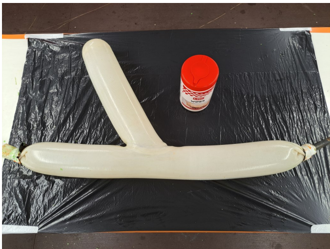
3. After cleaning, check the Bladder for damage.
