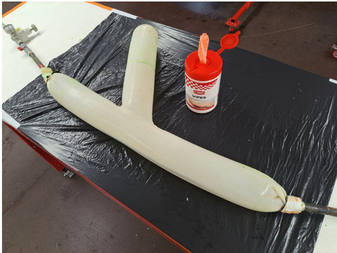
1. Add approximately 0.2 Bar (2.9 PSI) air to the Bladder.
