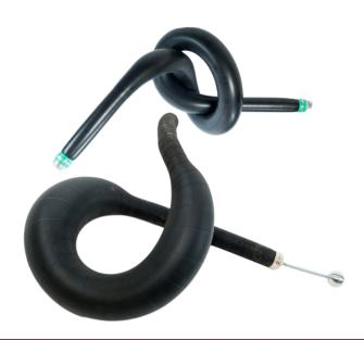
The Picote Bendy Packers are part of the Picote Pro Packer series and are designed for repairs in pipe bends. These Packers can be pushed through several bends to the renovation location through the innovative and patented Front-Wheel Drive System. This allows them to travel longer distances and easily navigate through multiple 90° bends.
