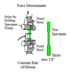
A piece of finished product, with a maximum thickness of .125-inches, is machined into a dog-bone shape. Each end of the test specimen is placed in opposite facing clamps which then attempt to pull it apart.
