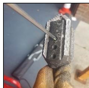
Tighten screws starting with the screw furthest away from the shaft end
