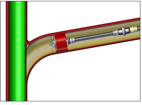
Step 2. Carefully drill the hole. Continue to push through so that you remove as much the liner away from the connection as possible. **Beware that you do not damage the already lined pipe during the process.** Use Smart Cutter™ grinding panels to grind the hole edges before removing the tool from the
