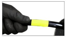
Attach a visual marker (tape) to the outer casing of the flexible shaft. Place it around half a metre from the end point of the shaft. The mark will indicate the chain's location and prevent possible injuries when the Pipe Cutter is removed from the pipe, including injury by rotating parts.
