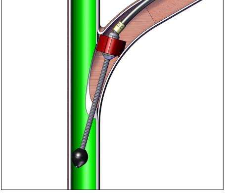
Step 3. It is recommended to use the lined Twister version when opening connections in already lined pipes. If Smart Cutter<sup>™</sup> with drill head is used, you will damage the lined pipe during the opening process. Select the Twister according to the size of host pipe, for the job. Drill the connection open carefully. Push the Twister
