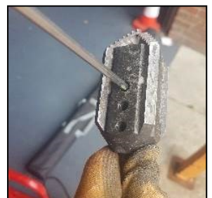
Tighten screws starting with the screw furthest away from the shaft end
