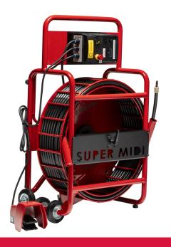
The Super Midi Miller is designed for cleaning, descaling, root removal, and cutting/reinstatements in DN70-150 (3-6") pipes. It has a range of 20m (65') that can be increased by an additional 10m (32') with a shaft extension. It can also be paired with the Picote Maxi Coating Pump to coat pipes DN70-200 (3-8").
