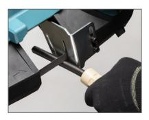
Always inspect the Flexible Shaft before each use. Run the machine for 30 seconds, in clockwise direction, to allow the shaft to return to its resting position. If there are potential weak points, or the shaft is damaged, cut off the damaged length using a bandsaw. For most tools, the shaft should extend ~40mm (1 ½") past the casing. Hubs and Original chains without a leader require more exposed shaft.
