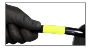
If not using a Leader, attach a visual marker (tape) on the outer casing of the Flexible Shaft. Place it around 500mm (20") from the end of the shaft. The marker will indicate the tool location and help prevent possible injury from the rotating parts by alerting you when the tool is about to exit the pipe.
