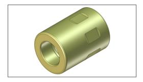
Always use a Sleeve when working with a Miller. It prolongs the lifetime of the Flexible Shaft and prevents the outer casing from melting in the tool end. Sleeves can be reused when the outer casing has been shortened.
